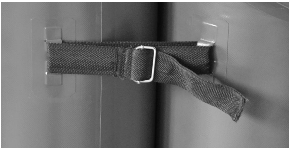
Connecting individual bunkers into a single structure using straps
